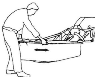
Fig. 9. Turning mower when moving from transport to working position and other way round.
