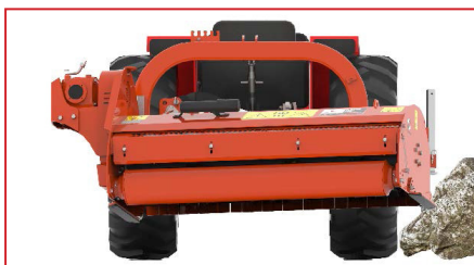
The Antishock system allows the machine to avoid any stones or obstacles during its cutting operation.
