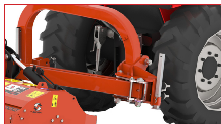
The Floating System allows the machine to follow the terrain surface profile during operation.
