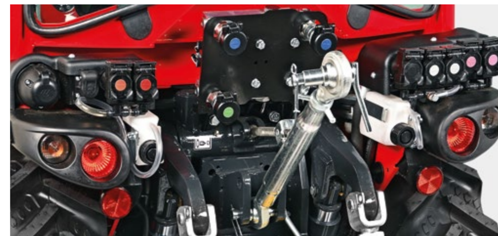
HYDRAULIC SYSTEM Modular hydraulic system with up to 11 hydraulic couplings divided into continuous flow, double acting and free return. All connections are served by hydraulic hoses with an increased cross-section to reduce pressure losses and thus improve the efficiency of the system.
