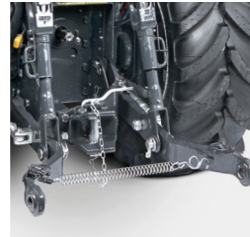
HYDRAULIC LIFT Adjustable lift arms; cat. 2 sliding quick hitches.
