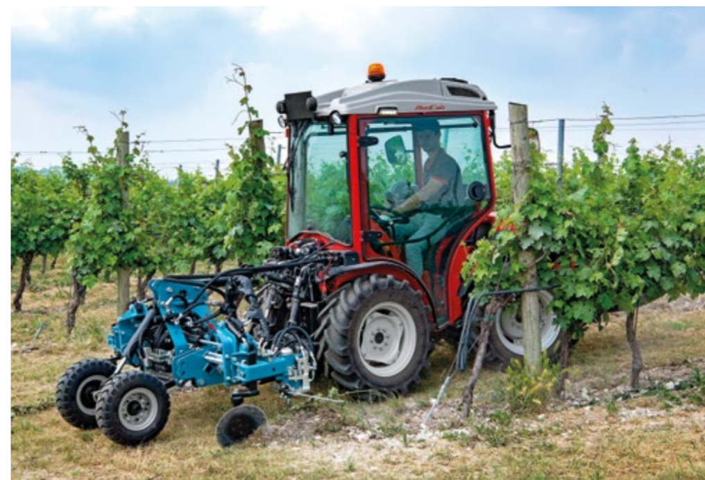
HYDRAULIC SYSTEM Modular hydraulic system with up to 11 hydraulic couplings divided into continuous flow, double acting and free return. All connections are served by hydraulic hoses with an increased cross-section to reduce pressure losses and thus improve the efficiency of the system.
